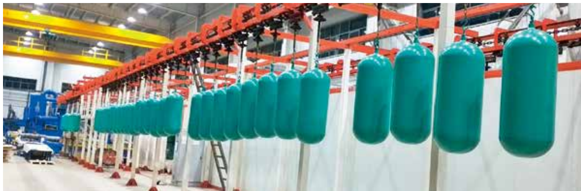
钢质无缝气瓶生产五车间喷涂工序
